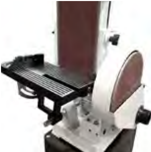
Tilttable belt from 0° to 90°
