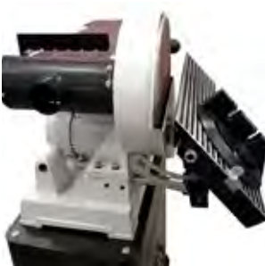
Tilttable table from 0° to 45°
